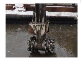
Durable, low-maintenance operation due to large-scale drive shaft bearing, heavy-duty sealing system and robust housing structure. Suitable for hard continuous running.
